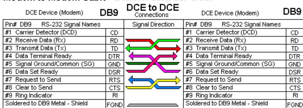
Note: Signal directions reversed if devices are DTE to DTE - "Null Modem" cable for DTE devices also connects pins #1 & #6 on each side to simulate Carrier (CD) which is required by some Terminal program software.
