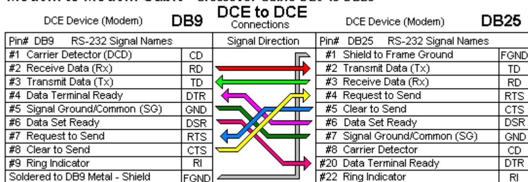
Note: Signal Directions Reversed if both devices are DTE but pin connections are the same.
