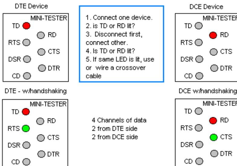
If the same light (TD or RD) is lit, use a crossover cable or null modem connector that swaps the connections for pins #2 and #3 and other pins as needed.
