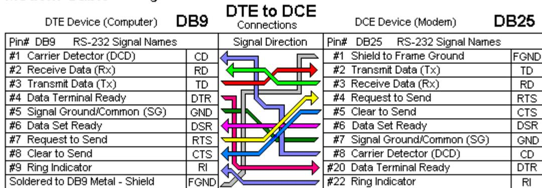
Note: Signal Directions Reversed when DB9 is DCE and DB25 is DTE
