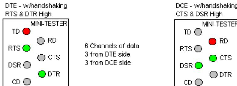
If the device is "port powered" check the active side, then plug in the port powered device and see if other (TD or RD) LED is lit. If not, try swapping the leads with a null modem cable, see if the other LED now lights. If not, you may not have enough voltage on the handshaking lines of the port to steal power from.
