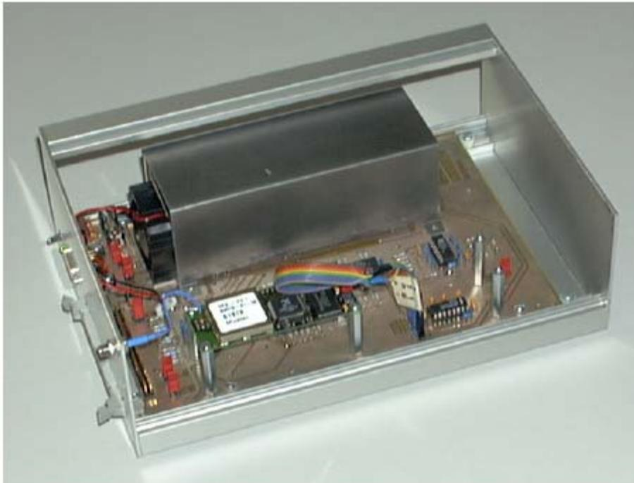
Figure 7: The Sensor Board with the Flow Channel and the Fan
