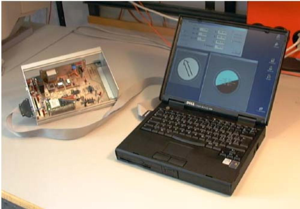
Figure 10: The Finished System with Laptop, Sensor Board and PCMCIA Measuring Card
