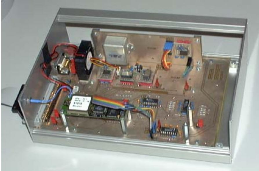
Figure 8: The Sensor Board with Individual Sensors
